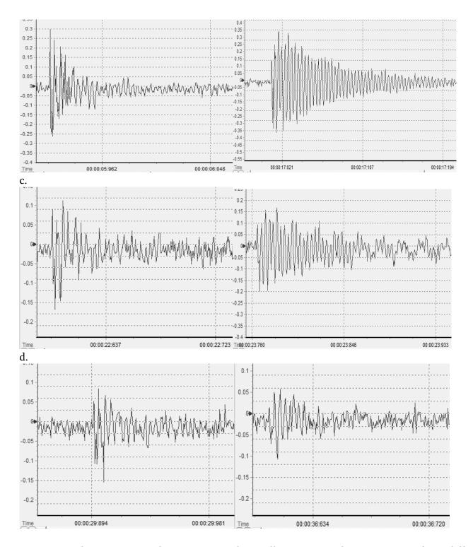
Fig.5. Recording acoustic pulses encountered in collisions on a plastic container from different distances: 1 column-sensitive sensor, 2 column-conventional sensor, a) Pendulum deviation of 25 cm, b) deviation of 20 cm, c) deviation of 15 cm, d) deviation of 10 cm; x-axis is time in sec, y-axis is the acoustic signal intensity in volts.
