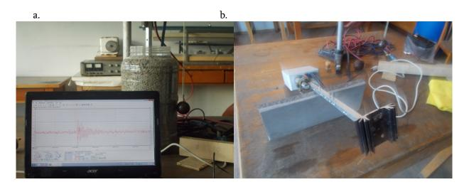
Fig.4. aexperimental equipment, b)acoustic sensor with fixed aluminum rod and radiator for increasing sensitivity
