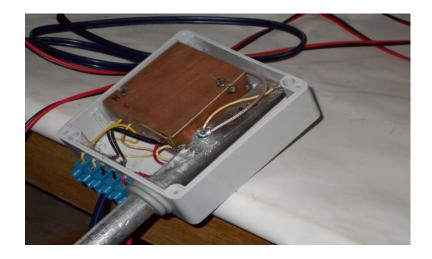
Fig.3. Acoustic sensors
