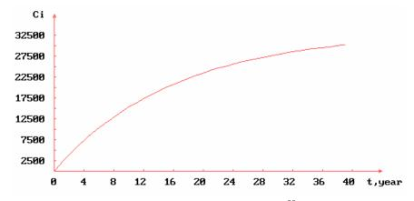
Fig. 4. Change in a time of activity of isotope  $Sr^{90}$  in the Black Sea, when the source was located on depth of 1205 m.
