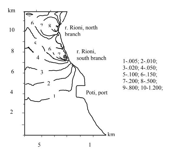
Fig. 10. Isolines of concentration of the Rioni alluvium ( $w_{G}=0.003$  cm/s) on depths of 1 m (in units kg/m<sup>3</sup>, February)
