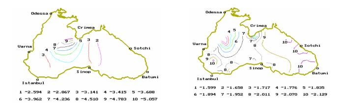
Fig. 5. Isolines of concentration of  $Sr^{90}$  (in unites of Bq/m3, the depth of the source location – 1205 m) on horizons: (a) – 1105 m, (b) – 85 m.
