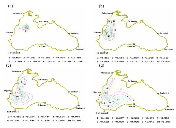
Fig.2. Isolines of the oil concentrations in the first numerical experiment (in unites of mg/l) at different moments after emergency oil emission: (a) - 2 days, (b) - 10 days, (c) - 15 days, (d) - 30 days.
