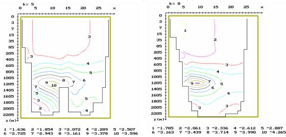
Fig. 6. Isolines of concentration of  $Sr^{90}$  (in unites of Bq/m3, the depth of the source location – 1205 m) on vertical sections zx.
