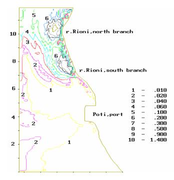
Fig.11. Calculated deformation of the sea bottom (in metres) caused by deposition of solid particles ( $w_G = 0.003 \text{ cm/s}$ ) during one year.
