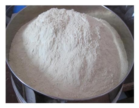
Fig. 3. Photo of AgI/nanosilica powdery reagent (LN-212).
