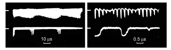
Fig.3. Periodically repeated orbital instability in magnetron  $r_a = 3.2cm$ ;  $r_c = 1.0cm$ ; L = 7cm; B = 1.2kG; V = 1.5kV;  $p = 6 \times 10^{-6}Torr$ .
