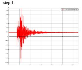
Fig. 5 - Uncorrected records of maximum horizontal components of earthquake (07.06.2017)
