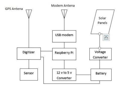
Fig. 2. Block diagram of stations
