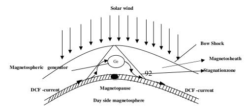
**Modeling of the magnetopause in kinematic approximation**. Thus, due to the change in the DCF- surface current contour curvature a dynamo-effect takes place the focal area. It means that intensity of the magnetic field increases in a certain segment of the magnetopause. To some extent the dynamo-effect makes the magnetospheric generator work, which transforms the solar wind energy into the DCF-current energy.
