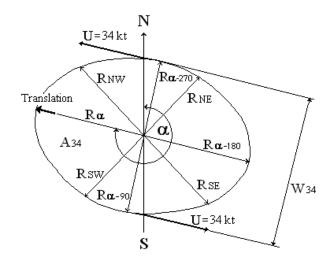
Fig. 2. The scheme of non-circular TH:  $A_{34}$  - area inside tangent velocity 34 kt (17.5 m/s);  $R_{NE}$ ,  $R_{SE}$ ,  $R_{SW}$  and  $R_{NW}$  - TH radii at tangent velocity 34 kt in Northeast, Southeast, Southwest and Northwest quadrants, respectively;  $\alpha$  - TH translation azimuth;  $W_{34}$  - TH transverse size at tangent velocity 34 kt.
