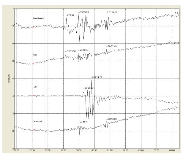
Fig. 4. WL oscillations due to passage of wave-trains of the Chile earthquake 16-09-2015,time:22:54,M8.3.Reactions successively from top to bottom in: Nakalakevi, Gori, Oni,Marneuli.
