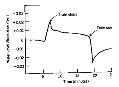
Fig. 2. Water level response to train passing close to a well
