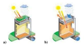
Photo 14. Water amount in the drainage system:a) in case of green coverage; b)in case of traditional roofing
