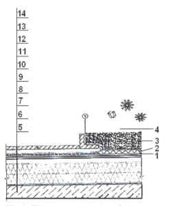
Fig. 1. The cover construction of greenery: 1 – geotextile 350-400 g / m<sup>2</sup>; 2 - Planter life; 3 - ground; 4 - Greening; 5 - roofing tile; 6 - Steam insulation; 7 - hitter; 8 - reinforced cement-sand crust; 9 - bitumen primer; 10 –hydro isolation 2 layer; 11 -plastic layer;12 - Drainage component; 13 - reinforced cement-sand crust; 14 - sidewalks or floor tiles
