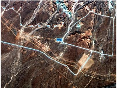
Fig. 1. ER-2/AVIRIS hyperspectral aerial image Mojave (USA) power station, September 6, 2018, pseudo-natural color composite, spectral bands 36 (684 nm), 20 (550 nm), and 10 (453 nm), GSD 5.8 m
