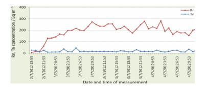
Figure 4. Radon and thoron concentrations in the basement of the private house Melikadze
