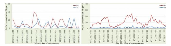
Figure 3. Radon and thoron concentrations in the Turkish bath (ground floor) in Tbilisi and in the basement of the Institute of Geophysics in Tbilisi
