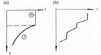
Fig. 1. Temperature distribution in the upper layer of the ocean:(a) schematic profile of temperature: (1) is the upper uniform layer,(2) is the upper thermocline [16]; (b) precise measuring profile [17].
