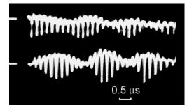
Fig.13. Orbital instability in magnetron  $r_a = 3.2cm$ ;  $r_c = 1.0cm$ ; L = 7cm; B = 1.2kG; V = 1.5kV;  $p = 5 \times 10^{-6}Torr$ .
