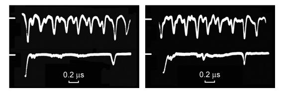
Fig.9. Approach of vortex structures in magnetron  $r_a = 3.2cm$ ;  $r_c = 1.0cm$ ; L = 7cm; B = 1.5kG; V = 1.5kV;  $p = 1 \times 10^{-4} Torr$ .
