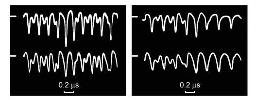
Fig.8. Approach and merging of vortex structures in magnetron  $r_a = 3.2cm$ ;  $r_c = 1.0cm$ ; L = 7cm; B = 1.5kG; V = 1.5kV;  $p = 1 \times 10^{-4} Torr$ .
