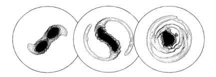
Fig.10. Merging of vortex structures [9].  $D/2R_{\nu} = 1.48$ ,  $t = 10,40, and 70 \mu \sec$
