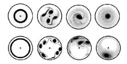
Fig.7. Time evolution of an electron rings [13] Top:  $(r_i/r_a) = 0.5$ , t = 0.01, 3, 10, 30ms. Bottom:  $(r_i/r_a) = 0.79$ , t = 0.01, 1, 5, 30ms.
