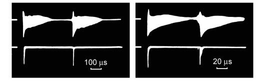
Fig.3. Diocotron instability and vortex structures in inverted magnetron [4]  $r_a = 1.0cm$ ;  $r_c = 3.2cm$ ; L = 7cm; B = 1.8kG; V = 0.9kV;  $p = 2 \times 10^{-6}$ ,  $1 \times 10^{-5} Torr$ .
