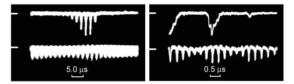
Fig.14. Orbital instability and electron ejection in magnetron  $r_a = 3.2cm$ ;  $r_c = 1.0cm$ ; L = 7cm; B = 1.2kG; V = 1.5kV;  $p = 5 \times 10^{-6}Torr$ .
