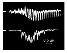
Fig.5. Vortex structure formation and ejection of electrons in inverted magnetron [3]  $r_a = 2.0cm$ ;  $r_c = 3.2cm$ ; L = 7cm; B = 1.5kG; V = 1.0kV;  $p = 1 \times 10^{-5}Torr$
