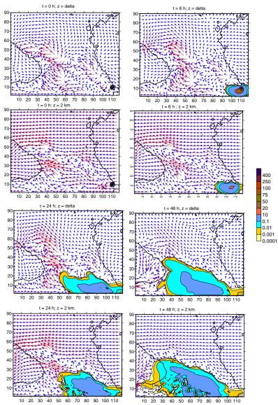
Fig. 4. The spatial distribution of the concentration C(a.u.) of the passive pollution substance emitted in the vicinity of t. Baki t = 0, 6, 24 and 48 h on the atmosphere surface level  $z = \delta(x, y)$  and z = 0 in case of the background eastern wind.
