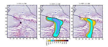
Fig. 3. The spatial distribution of the concentration C(a.u.) of the passive pollution substance emitted in the vicinity of t. Poti in t = 0, 24 and 48 h on the atmosphere surface level  $z = \delta(x, y)$  in case of the background northern wind.
