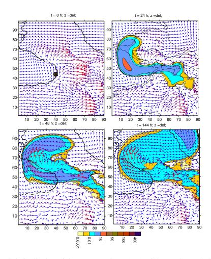
Fig. 2. The spatial distribution of the concentration C(a.u.) of the passive pollution substance emitted in the vicinity of t. Poti in t = 0, 6, 24 and 48 h on the levels  $z = \delta(x, y)$  and 2 km in case of the background western wind.
