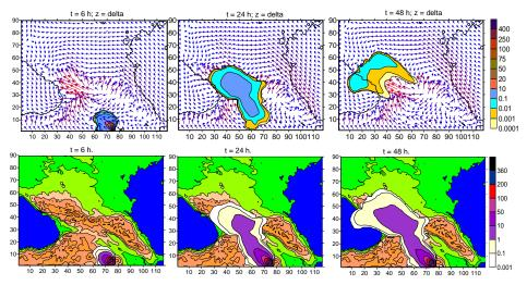
Fig. 7. The spatial distribution of the concentration in the atmosphere surface layer (upper row) and surface density of the sediment on the earth (lower row) of the radioactive pollution  $I^{131}$  (a.u./m<sup>2</sup>) at t = 0, 24 and 48 in case of the background south-east wind.
