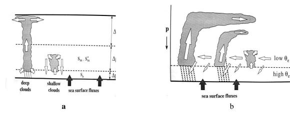
Fig. 6. Vertical structure of Emanuel's hurricane model: "(a) - deep clouds transfer mass from the subcloud layer to the top layer; **shallow clouds** exchange entropy between the lower troposphere and the subcloud layer without producing a net mass flux; (b) illustration of airflow in a developing Emanuel's tropical cyclone model; for a cyclone to spin up, lower tropospheric
