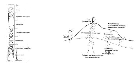
fluid; bubble; bubble-slug; slug; slug-annular; annular; dispersed-annular; drops; vapor. Approximate sequence flow structures in vertical evaporator tube [9].
